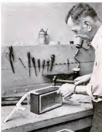
Applying strips of lead to the miniature chest. Below are the drawings
